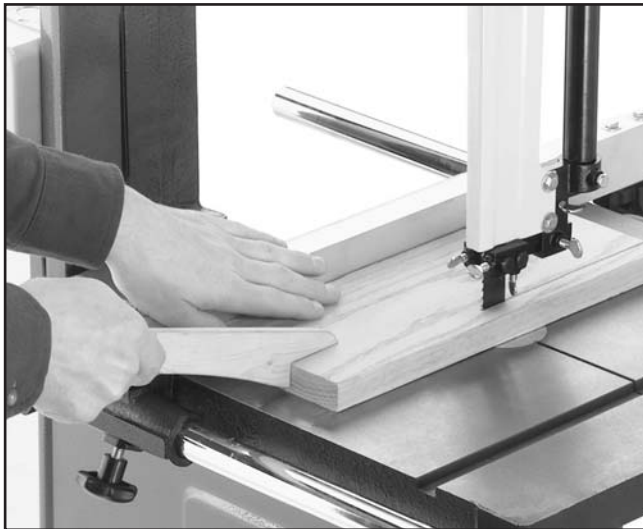
Figure 41. Ripping with a push stick.
